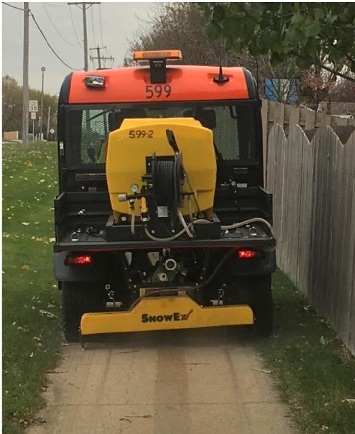
**Five anti-icing units can be deployed – four on roadways and the newest UTV unit for sidewalks and Village properties (pictured here)**
